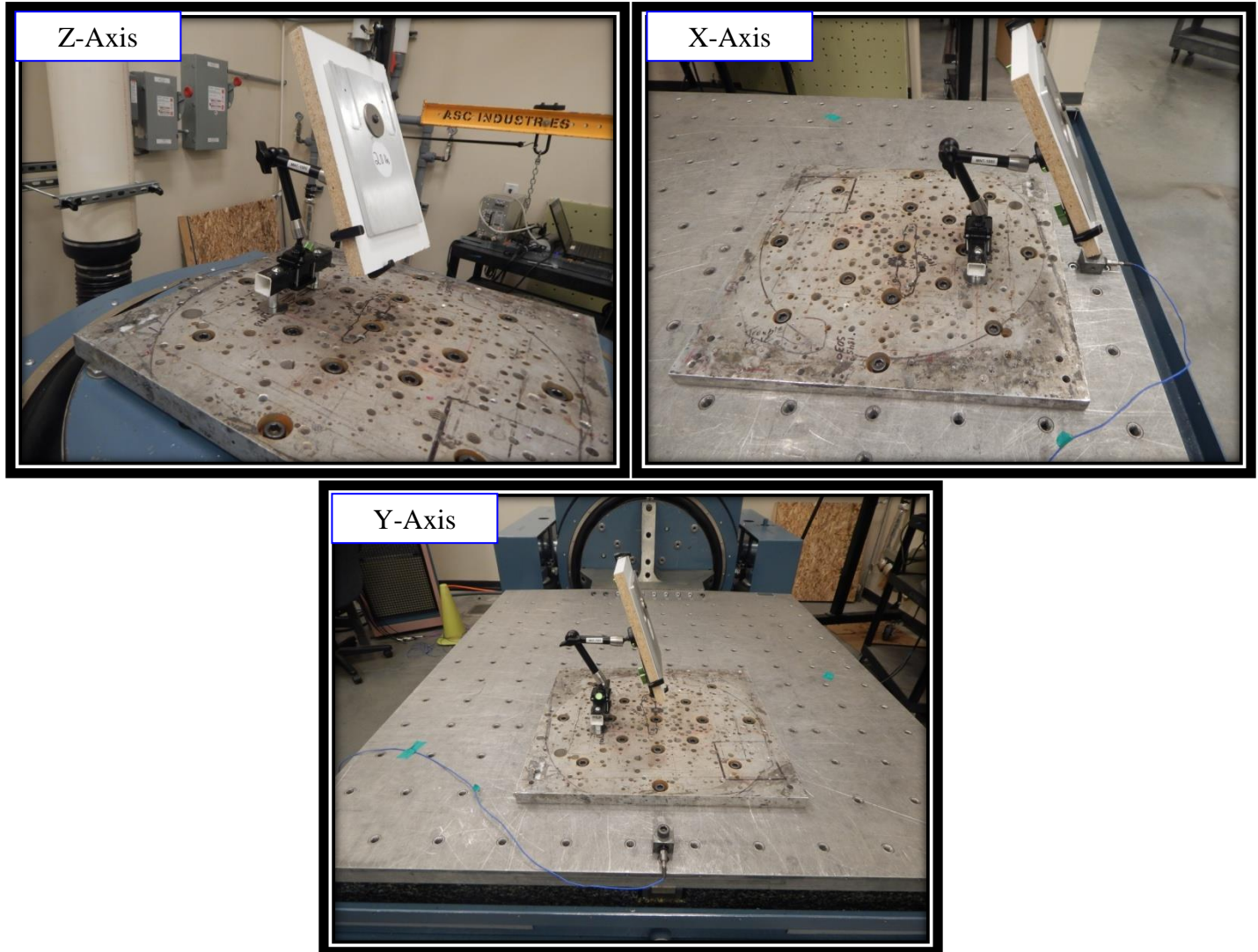
Figure 6: View of test setup for MNT-1880- (Airbus Square Tube Mount)
